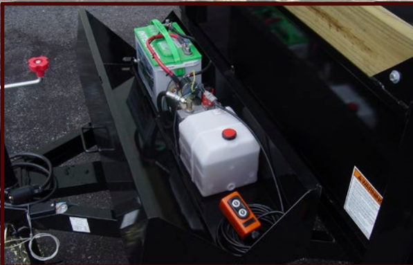
Pump & Battery Box
