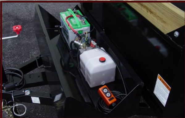
Pump & Battery Box
